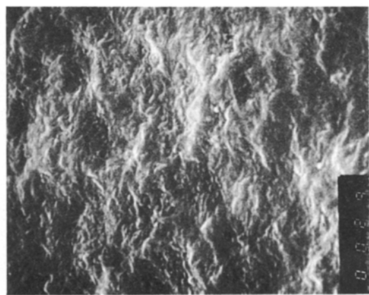
Figure 18 “Dissolved” groove from acid-treated monofilament, draw ratio 1:1, \times 3200 .
